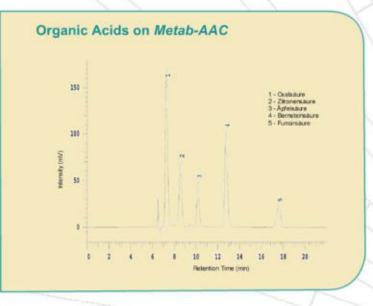
The separation occurs on a robust polystyrene-divinylbenzene (PS-DVB) phase which is stable between pH 0 and pH 14 and at temperatures from 5 to 90°C.
